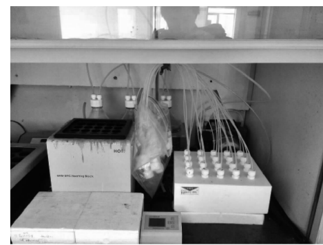
图 1 真空赶酸系统装置图 Figure 1 Vacuum acid system installation drawing
